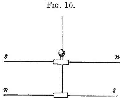
It must be so arranged that one of the needles shall be within the coil through which the current flows, while the other needle swings freely above the coil, the vertical connecting piece passing through an appropriate slit in the coil. Were both the needles within the coil, the same current would urge them in opposite directions, and thus one needle would neutralise the other. But when one is within and the other without, the current urges both needles in the same direction.
