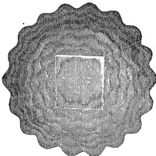
matters are here so arranged, that the vapour shall issue laterally; and it sometimes happens that the escape is rhythmic; the vapour issues in regular pulses, and then we have our drop of water moulded to a most beautiful rosette. It is there now—a round mass of liquid, two inches in diameter, with a beautifully crimped border. Throwing the beam of the electric lamp upon this drop, so as to illuminate it, and holding this lens over it, I
