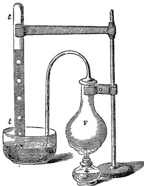
tube *t t*. The air speedily depresses the coloured liquid, until now, in the course of a very few seconds, the whole column of liquid has been superseded by air.
