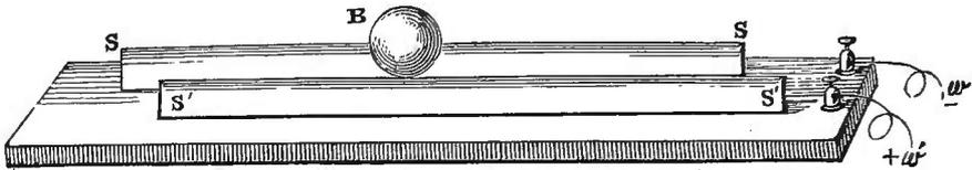
produces an elevation of the rail at these points. Observe the effect: the ball, which a moment ago was tranquil, is now uneasy. It vibrates a little at first without rolling; now it actually rolls a little way, stops, and rolls back again. It gradually augments its excursion, now it has gone farther than was intended; it has rolled quite off the rails, and injured itself by falling on the floor.
