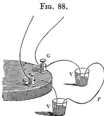
between the two vessels, part of the current will pass through this wire and return to the pile. The quantity of electricity circulating in the galvanometer will be thus diminished, and with it the deflection of the needle.
