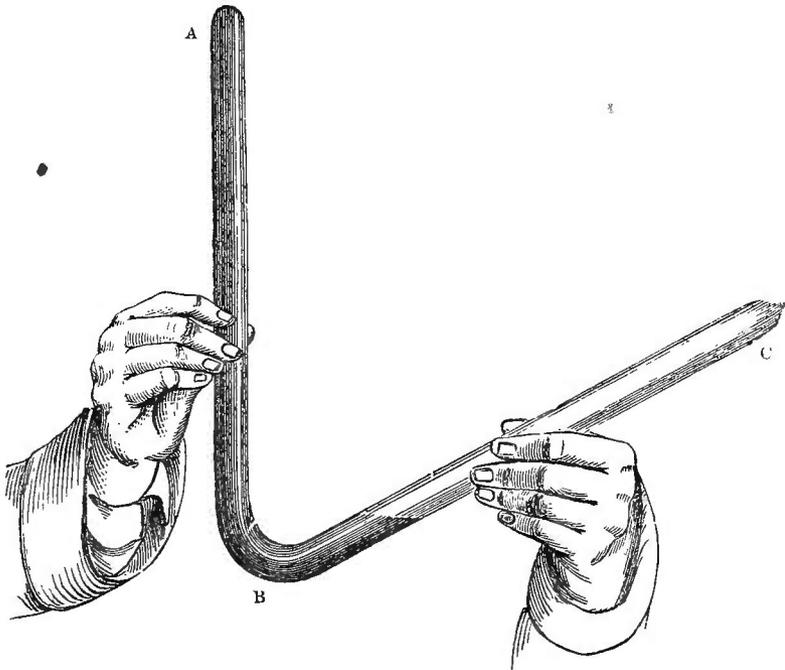
in true contact with the interior surface of the tube. As the tapping continues you notice an alteration in the sound; the jingling has now disappeared, the impact being hard, like that of solid against solid. I now raise the tube, and turn the column of water upside down, but there it stands in the arm *A B*. Its particles cling so tenaciously to the sides of the tube, and lock themselves so firmly together, that it refuses to behave like a liquid body; it declines to obey the law of gravity.
