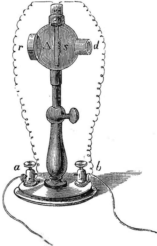
diameter. Behind the spiral, finally, is a metallic reflector, *r*, which augments the flux of heat without sensibly changing its quality. In the open air the red-hot spiral is a capricious source of heat, but surrounded by its glass globe its steadiness is admirable.\*
