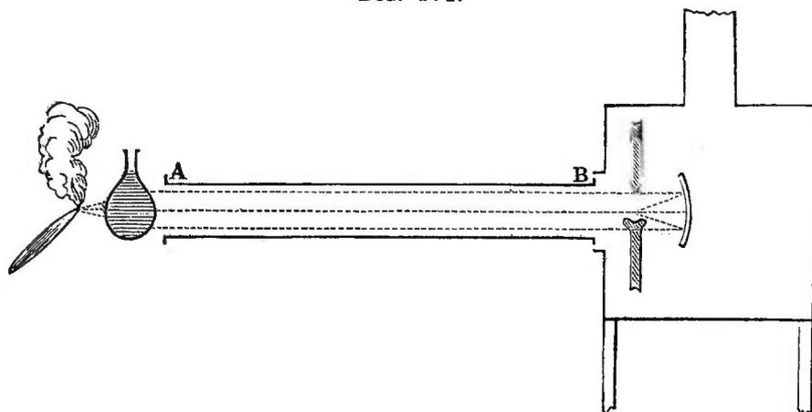
waste of radiant heat. Such a tube, placed in front of the camera, is represented at A B, fig. 104. The flask may be held against its end by the hand, or it may be permanently fixed there. With a battery of fifty cells, platinum may be raised to a white heat at the focus of the flask.
