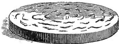
the ceiling, and produce the effect which you are now to witness. Pointing the rod which unites the plates, in the direction of the paper drum, I draw the resined rubber vigorously over the rod: a single stroke has caused the sand to spring into a reticulated pattern. A precisely similar effect is produced, by sound, on the drum of the ear; the tympanic membrane is caused to shiver, like that drum-head of paper, and its motion, conveyed to the auditory nerve, and transmitted thence to
