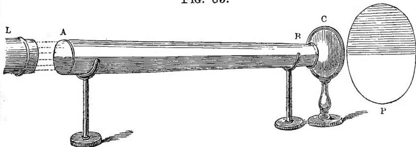
here arranged which will show you that this pellucid liquid, in sufficient thickness, has a very decided colour. This tube A B (fig. 83), fifteen feet long, is placed hori-
