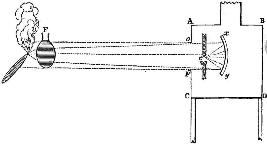
$o p$  the aperture in front of the camera, through which issues the beam reflected by the mirror  $x y$ .
