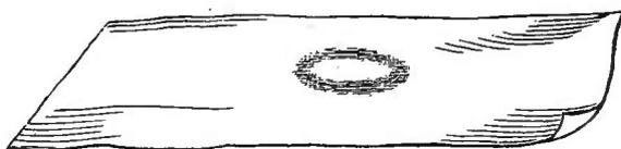
candle, we have a charred ring upon the paper (fig. 18). Operating in the same manner with a jet of gas, we obtain the ring which it produces. Within the ring the paper is intact, for at this place the unburnt vapour of the candle, or the unburnt gas of the jet, impinges against the surface, and no charring can occur.
