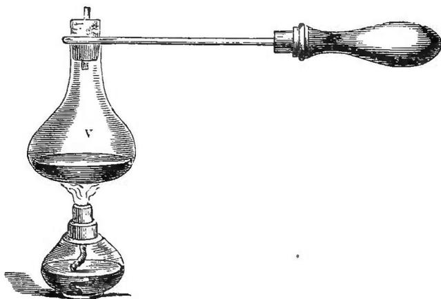
they actually come into operation. The effect of a sudden generation of steam has been illustrated by an experiment which may be made in your presence. Here is a copper vessel, v (fig. 50), with a neck stopped with a cork,
