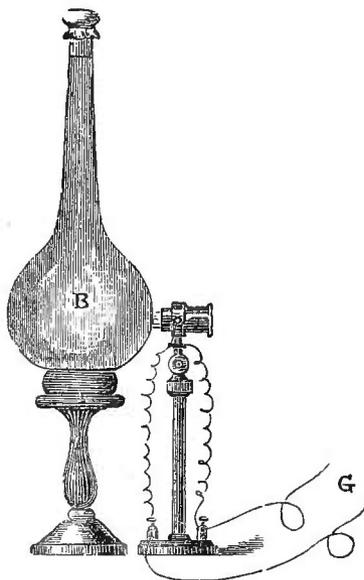
the liquid in front of the pile, but you see it approaching. The salt is now solidified opposite the pile; and mark the effect. The atoms, in falling to the solid form, develop heat; this heat communicates itself to the glass envelope, which, in its turn, warms the pile, and the needle flies to  $90^\circ$ . The quantity of heat thus rendered sensible by solidification is exactly equal to that which was rendered latent by liquefaction.
