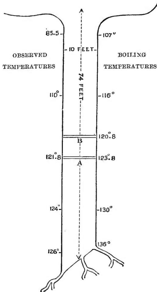
below is further relieved. More steam is generated; from the middle downwards the mass suddenly bursts into ebullition: the water above, mixed with steam-clouds, is projected into the atmosphere, and we have the geyser eruption in all its grandeur.
