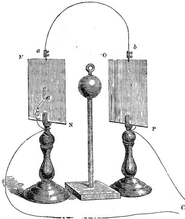
(344) Exactly midway between the two sheets of tin, is set a stand on which is placed a heated copper ball; the ball radiates against both sheets: on the right, however, the rays strike upon a coated surface, while on the left they strike upon a naked metallic one. If both surfaces absorbed equally the radiant heat—if both accepted with equal freedom the motion of the ethereal waves—the bismuth junctions at the backs would be
