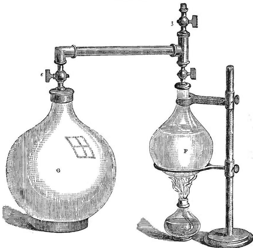
dually becoming less through its own slow condensation. I hasten the condensation by pouring cold water on the flask; the bubbles are more copiously generated. By plunging the flask bodily into cold water we might cause it to boil violently. The water in F is now at rest, and some degrees below its ordinary boiling point. I turn the cock *e*, which opens a way for the escape of the vapour into the exhausted vessel G; the moment the pressure is dimi-
