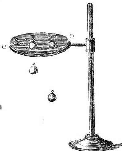
with different velocities. The iron and the copper are working themselves much more vigorously into the fusible mass than the others; the tin comes next, while the lead and the bismuth lag entirely behind. And now the iron has gone clean through; the copper follows; the bottom of the tin ball just protrudes from the lower surface of the cake, but it cannot go farther; while the lead and bismuth have made but little way, being unable to sink to much more than half the depth of the wax.
