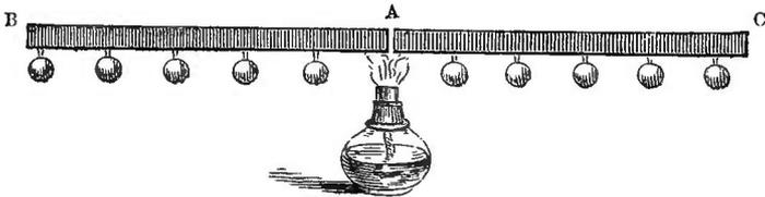
attached by wax at equal distances from the place of junction. Under the junction is placed a spirit-lamp, which heats the ends of the bars: the heat will be propagated right and left through both. The bar A B is iron, the bar A C is copper; the heat travels to a greater distance along the copper, which is the better conductor, and therefore liberates a greater number of its balls.
