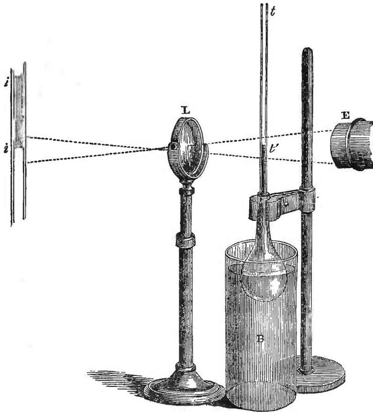
the expansion of the liquid soon exceeds that of the glass, and the column rises. Two things are here illustrated: the expansion of the solid glass by heat, and the fact that the observed dilatation of the liquid does not give us its true augmentation of volume, but only the difference of dilatation between itself and the glass.
