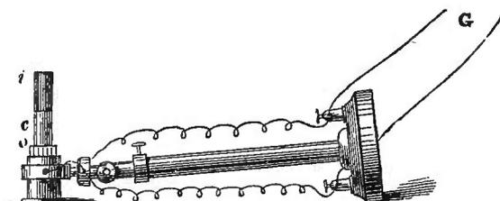
inches in height; this cylinder is to be my source of heat. Laying the thermo-electric pile, *o* (fig. 56), thus flat, with its naked face turned upwards, I place upon that face a cylinder of copper, *c*, which now possesses the temperature of this room. We observe no deflection of the galvanometer. I now place the warm cylinder, *i*, having first dried it, upon the cool cylinder, which is supported by the
