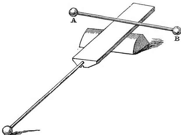
at  $M$ . We will heat the rocker to a temperature somewhat higher than that of boiling water, and lay it on a block of lead, allowing its knob to rest upon the table. You hear a quick succession of forcible
