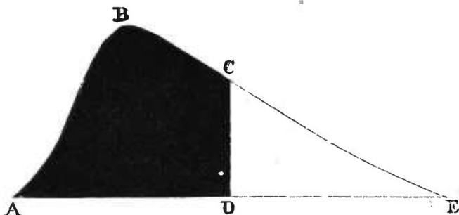
the distribution of heat in the solar spectrum. The results of his observations are rendered graphically in fig. 98, where the area **D C E** represents the visible, and **A B C D** the invisible radiation.
