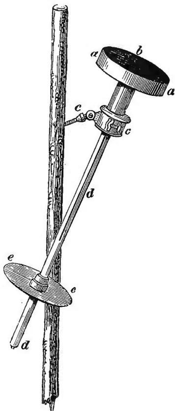
made at considerable heights. It is necessary that the surface which receives the sun's rays should be perpendicular to them, and this is secured by attaching to the brass tube which shields the stem of the thermometer, a disk, *ee*, of precisely the same diameter as the steel cylinder, *aa*. When the shadow of the cylinder accurately covers the disk, we are sure that the rays fall, as perpendiculars, on the upturned surface of the cylinder.
