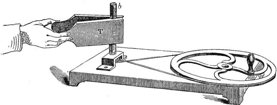
its conditions. We cannot devote two hours and a half to a single experiment, but I hope to be able to show you substantially the same effect in two minutes and a half. Here is a brass tube (*b*, fig. 3), four inches long, and of three-quarters of an inch interior diameter. It is stopped at the bottom, and screwed on to a whirling
