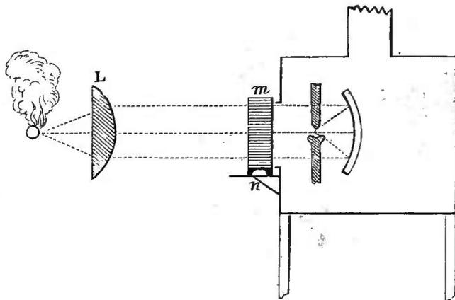
the coal-points are ignited, explosion, combustion, or calorescence, as the case may be, occurs at the focus.
