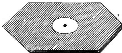
a crystal of quartz—forming a hexagonal pillar, which, if complete, would be terminated by two six-sided pyramids. That heat travels with greater facility along the axis of this crystal than across it has been proved in a very simple manner by M. de Senarmont. Of these two plates
