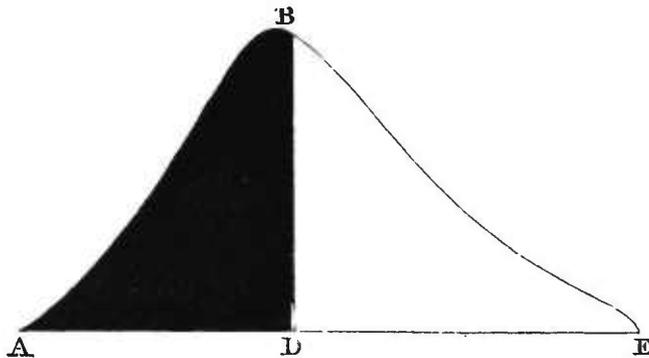
of a certain length be taken to represent a rise of one degree, a line of twice that length will represent a rise of two degrees, while a line of half the length would represent a rise of half a degree. In order to show the distribution of heat in the spectrum of the sun, Sir William Herschel adopted this device of representing temperatures by lines. Drawing a horizontal line A E, fig. 97, to represent the length of the spectrum, and erecting at its various
