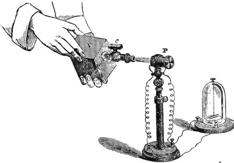
was not my object to draw upon the heat developed by my muscles; after condensation, therefore, the vessel was allowed to rest till all the heat generated by the condensation was dissipated, and the temperature of the air within and without the vessel was the same. When, therefore, the air rushed out, it had not the heat to draw upon which had been developed during compression. The heat from which it derived its elastic force was only sufficient
