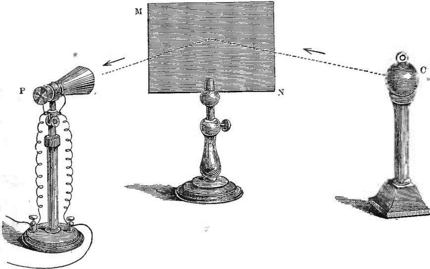
from the ball rebound from it, and strike the pile, and you observe the consequent prompt motion of the needle.
