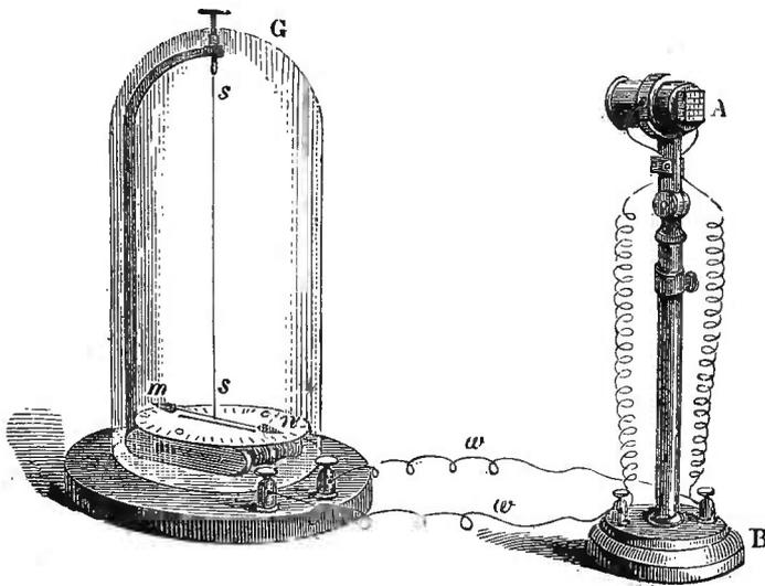
shade, *G*, from all disturbance by currents of air. To one end of the needle is fixed a piece of red, and to the other end a piece of blue, paper. All of you see these pieces of paper, and when the needle moves, its motion will be clearly visible to the most distant person in this room. This instrument is called a *galvanometer*.†
