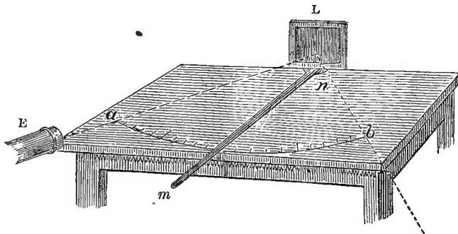
the mirror is a long straight lath, *m n*, so that the mirror, resting upon rollers, can be turned by the lath, which is to serve as an index. Those in front may see that the lath itself and its reflection in the mirror now form a straight line, which proves that the lath is perpendicular to the mirror. Right and left of the central line, *m n*, the arc is divided into ten equal parts; commencing at the end
