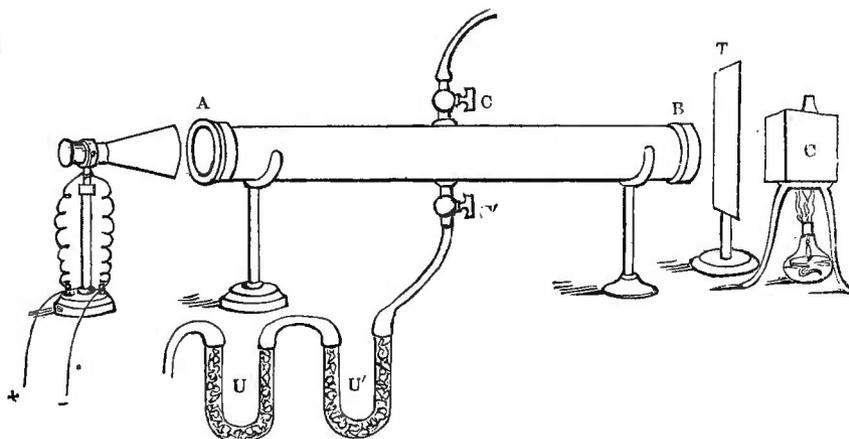
which, by means of the caps A and B, can be screwed airtight on to the ends of my cylinder.\* This is provided with two stopcocks, one of which, C, is connected with an air-
