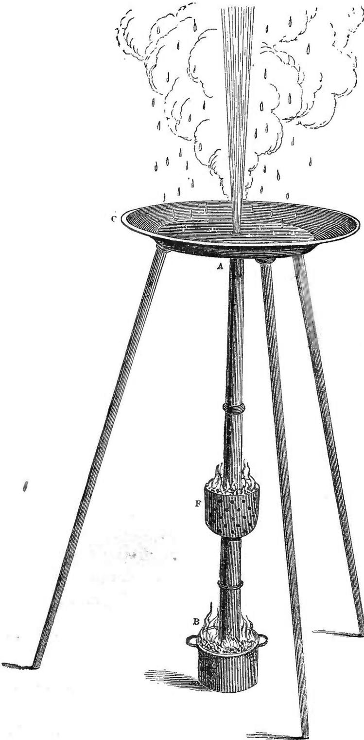
impetuous steam-gushes follow each other in quick succession, the water being squirted in jets fifteen or twenty feet high. These experiments prove that the geyser tube itself is the sufficient cause of the eruptions, and we are relieved from the necessity of imagining underground caverns filled with water and steam, which were formerly regarded as necessary to the production of these wonderful phenomena.
