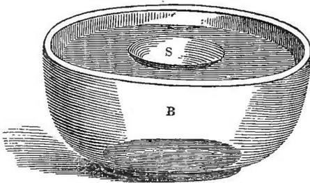
might naturally reply, that the basin will impart its heat instantly to the water, and be cooled down to the temperature of the latter. But nothing of this kind occurs. The silver for a time develops a sufficient amount of vapour under-
