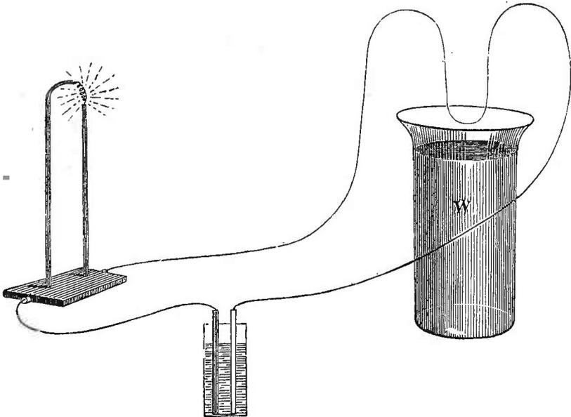
(253) Thus, then, I plunge the red-hot wire into a beaker of water *w* (fig. 59): the lamp immediately becomes almost too bright to look at. When the wire is raised out of the water, and the heat is allowed once more to develop
