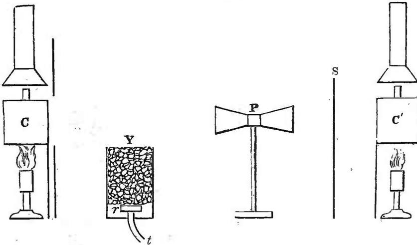
emergence of the saturated air from the cylinder, the needle moved and took up a final deflection of 5 degrees. The direction of the deflection showed that the opacity of the space, between the source *c* and the pile, was augmented by the saturated air.
