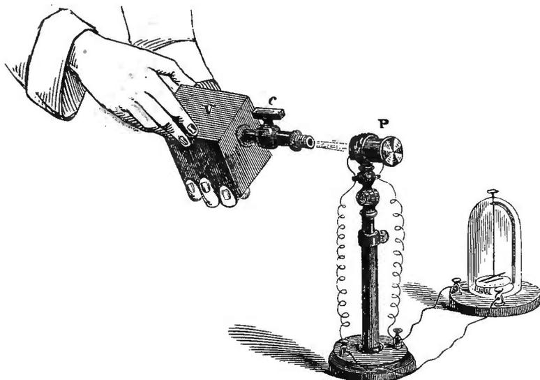
of air from the vessel *v* to strike against the face of the pile *P*. The magnetic needle instantly responds; its red end is driven towards me, thus declaring that the pile has been *chilled* by the current of air.
