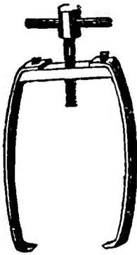
FIG. 193.—Cheap Press for heading-up Apple-Barrels.
