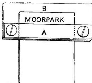
FIG. 187.—Device for Stamping Lead Tags.
