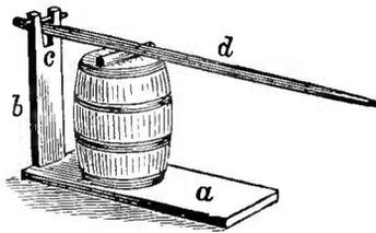
FIG. 192.—Simple Contrivance for heading-up Apple-Barrels.
