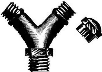
FIG. 266.—Y-Fixture for Vermorel Nozzles.
