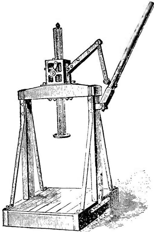
FIG. 194.—Press for heading-up Apple-Barrels.
