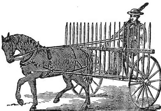
tached to a journal at the centre of the rake-head. By means of cams, stop, and spring, the lever and head are entirely at the will of the operator. A slight pressure, equal to seven or eight pounds, on a lever, causes the rake to revolve; and it is also readily elevated for backing, or for passing obstructions.
