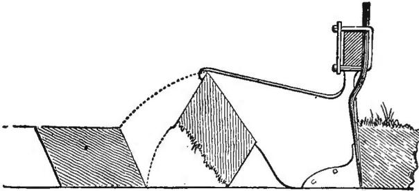
*The Inclined Cutter, Laying Flat Furrows.*
