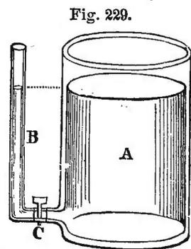
the tube, B, be now filled to an equal height, the same force will be exerted against the other side. To prove this, let the stop-cock be opened, when the two columns of water will remain at an exact level.
