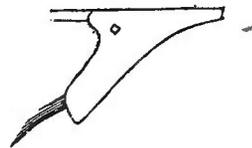
wise work well are hard to draw because the edge, being made too thick or obtuse, raises the earth abruptly. Fig. 124.
