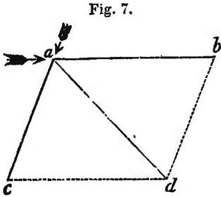
direction shown by the two arrows, and if one force be just sufficient to carry it from  $a$  to  $c$ , and the other to carry it from  $a$  to  $b$ , then it will move intermediate between the two, in the direction of the diagonal of the parallelogram  $a d$ , and to a distance just equal to the length of this diagonal or cross-diameter.
