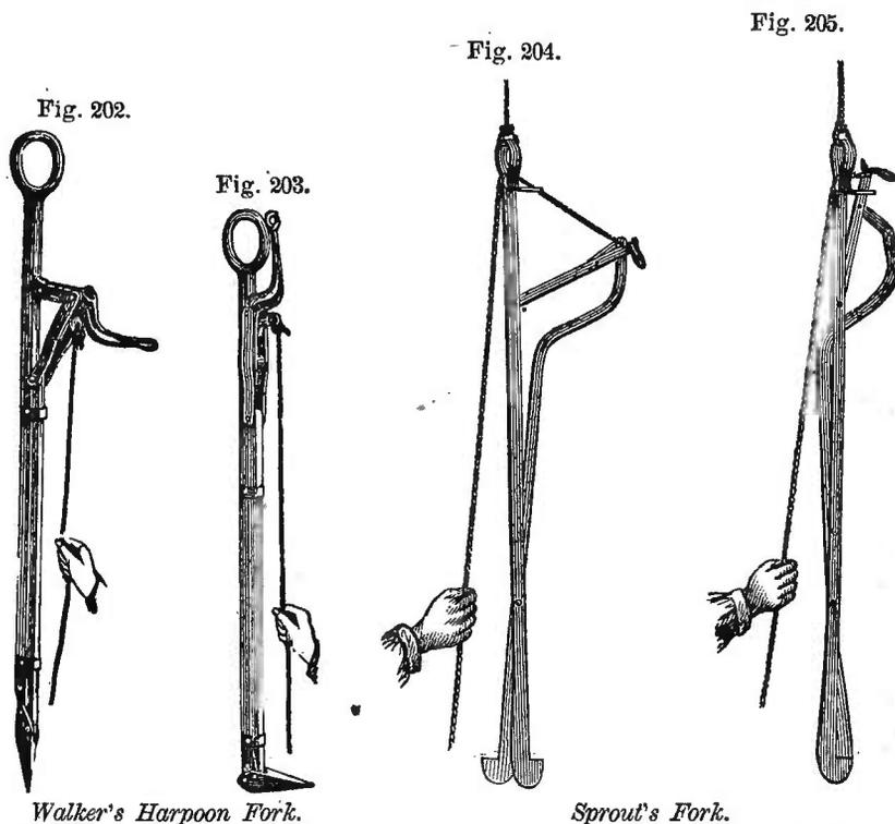
short straw. *Walker's* harpoon, made by Wheeler, Melick & Co., Albany, is a straight bar of metal, appearing almost as simple as a crow-bar, (fig. 202. Its point is driven into the hay as far as desired, when a movement at the handle is made, which turns up the point at right angles, (fig. 203,) enabling it to lift a large quantity of hay. A modification has spurs, which are thrown out on opposite sides. The combined fork and knife invented by Kniffen & Har-
