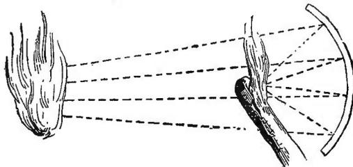
beating it out concave so as to fit a regularly curved gauge. If a foot in diameter, and carefully made, it will condense the rays of heat so powerfully at the focus, when held several feet from the fire, as to set fire to a pine stick or to flash gunpowder (fig. 294).
