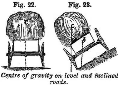
or it will immediately be thrown over by its own weight. A heavily and evenly loaded wagon on a level road will be perfectly safe, because the line of direction falls equally between the wheels, as shown in fig. 22, by the
