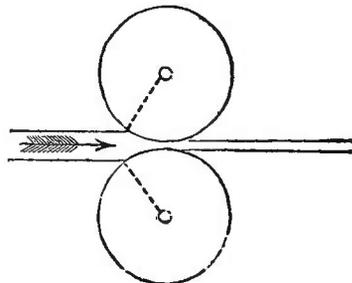
*Principle of the knee-joint in the rolling-mill.*
