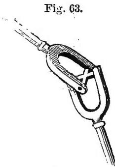
municated by means of the *universal joint*, as shown in fig. 63. This is commonly used in the thrashing-machine, where there is a slight change in the direction of motion between the horse-power and the thrasher.
