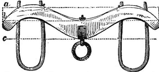
timber as wide as the dotted lines *a c*; and being thus weakened, it requires to be correspondingly large. Fig. 92 is equally strong, much lighter, and is easily made from a stick of timber only as wide as *a b* in the former figure.
