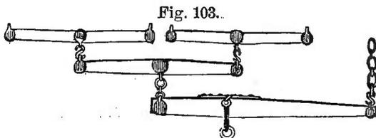
For these reasons, when only three horses are used, they should always be placed abreast. The force required for each may be rendered exactly equal by the whiffle-trees
