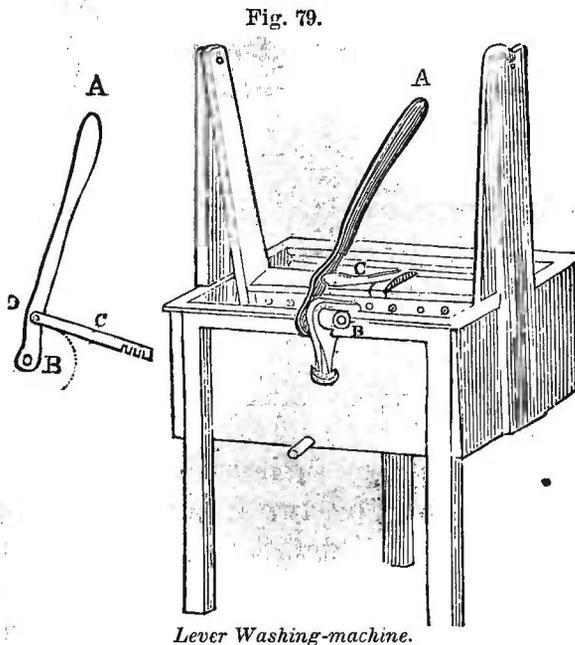
forated with holes, with great force against the clothes next to one side of the water-box. Like the printing-press, this machine exerts the greatest power just as the motion of the lever is completed, and at the time it is most needed. The same principle is exhibited in *Kendall's Cheese-press* (fig. 80), where the lever and the wheel and axle are combined with the two knee-joints, one on each side of the press, drawing down a cross-beam upon the cheese with a greatly multiplied power.
