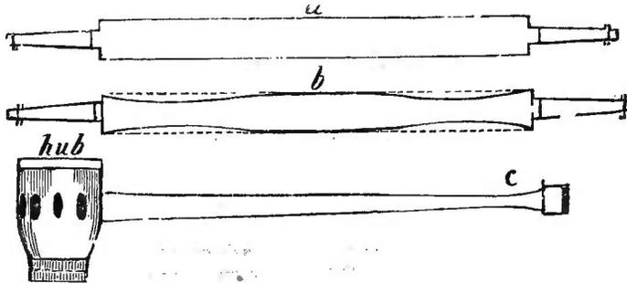
the outer ends, where they are soonest weakened by decay. Hence there should be nearly a uniform taper, slightly larger at the middle, and with an enlargement at the outer end, as *c* (fig. 94).
