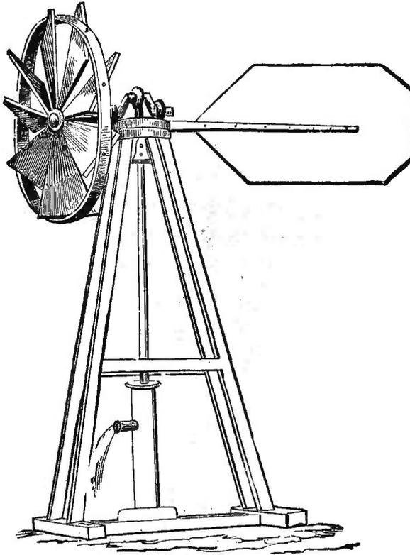
Wind-mills, like the preceding, which have fixed sails, *should not be more than three or four feet in diameter*, and even then will require care in storms. If larger, they will become broken by severe winds. The remedy is either to move the sails by hand at every considerable change in the force of the current, which would require nearly constant attention; or to use the self-regulating machines, of which there have been several invented, some of which have proved useful and durable.
