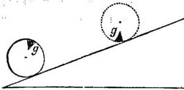
round ball, the centre of gravity will be exactly at the centre of the globe; if it be a rod of equal size, it will be at the middle of the rod. If a stone or any other substance rest on a point directly under the centre of gravity, it will remain balanced on this point; but if the point be not under the centre of gravity, the stone will fall toward the heaviest side.
