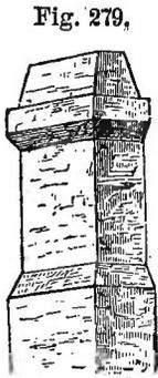
current at the moment of escape is swifter than below, and less acted upon by any downward blast of the wind, at the same time that the surface is smaller on which the wind can strike the current, as shown in fig. 278. A chimney of this character may be very easily made by contracting the tiers of brick, thus giving to it an ornamental appearance, as seen in fig. 279.\*
