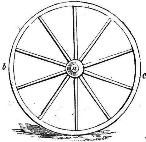
wheel will overcome twenty ounces of friction at the axle; or if the axle were twice as large, then, according to the same rule, it would require two ounces to overcome the same friction acting between larger surfaces.
