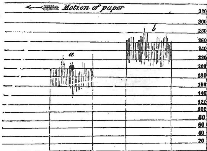
The markings of the Self-recording Dynamometer.
