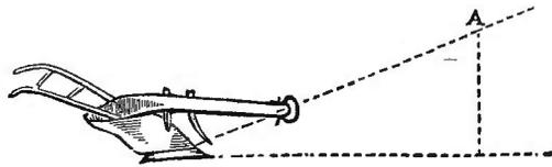
plow is necessarily thrown too much upon its point, to keep it from flying out of the ground, by which means it works badly in turning the furrow. In addition to this evil, the plowman is compelled to bear down heavily, adding to the friction of the sole on the bottom of the furrow, and greatly increasing his labor.
