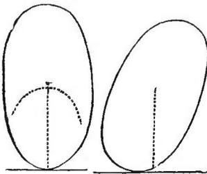
nearer the touching-point, that is, causes it to descend, and the body consequently falls over on its side. This may be easily illustrated with an egg, which will lie at rest upon its side, but falls when set on either end.
