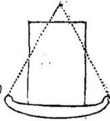
of the rockers is but little greater than the distance to the middle, *c*, as in fig. 39, the motion will be slow and gentle; but if this difference be greater, as in fig. 40, it will be rapid. When the centre is high, the rockers must have less curvature
