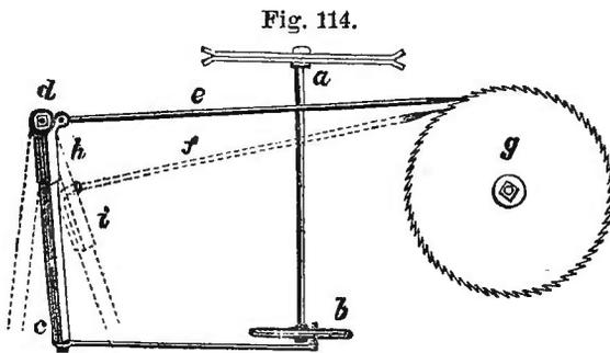
stated. In doing so, it causes the arm *d c*, to vibrate backwards and forwards, on a pin at *d*; the connecting rod *b c* being set near the circumference
