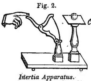
and heavy vessel; but the same force which sets a body in motion is required to stop it. Thus a wheel or a grindstone, made to revolve rapidly, would need as great an effort of the arm to stop it suddenly as to give it sudden motion. An unusual exertion of the team is necessary in starting a loaded wagon; but when once on its way, it would require the same effort of the horses to stop it as to *back* it when at rest.
