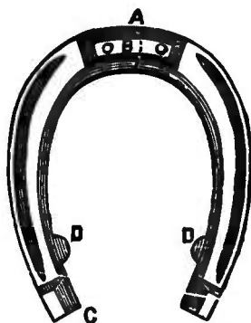
Fig. 74—Shoe for Contracted Feet.
