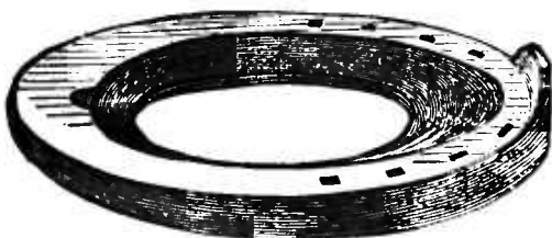
Fig. 118—Form of Shoe for Foundered Horses.
