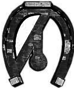
Fig. 131—A Form of Bar Shoe.
