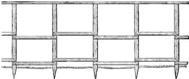
Fig. 38. Frame structure of the manure shed.
