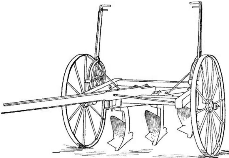
Fig. 23. A good gang-plow for shallow tilling.
