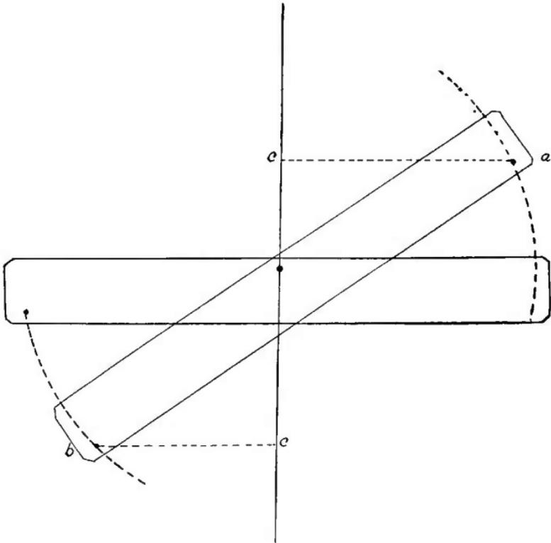
Fig. 22. Diagram showing the mechanics of the evener.
